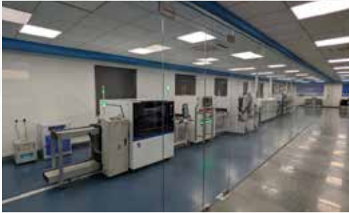
SMT Assembly Line in the BEST-Electronic Manufacturing Systems vertical at SASTRA University
