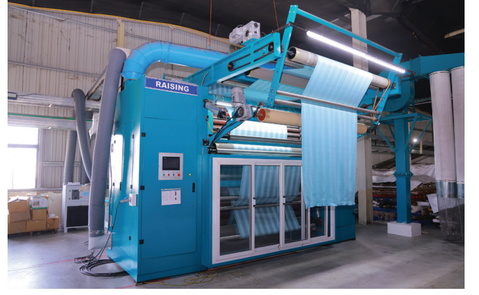
A view of new Raising Machine installed at our Fabric Division.
